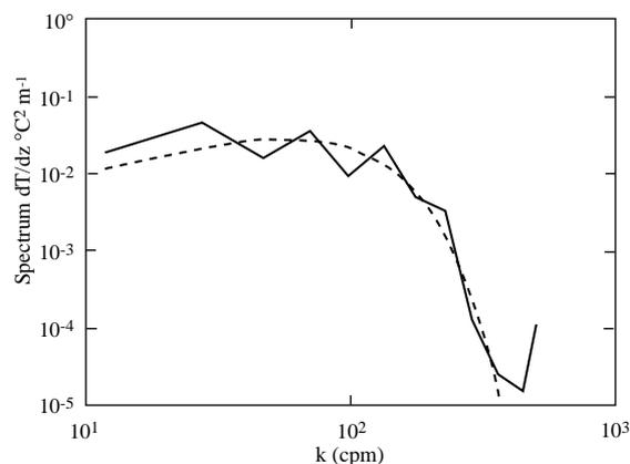
Figure 3. The wavenumber spectra of the temperature gradient signal and the fitted Batchelor spectra. The experimental conditions are,  $a = 3.1 \text{ cm}$ ,  $N = 0.615 \text{ rad/s}$ ,  $\alpha = 32.5^\circ$  and  $\beta = 10.2^\circ$ .
