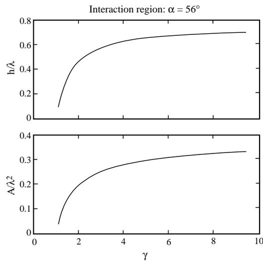
Figure 2. The variation of (a) the non-dimensional extent of the interaction area ( $h/\lambda$ ) and (b) the non-dimensional area ( $A/\lambda^2$ ) of the interaction region with  $\gamma$ .
