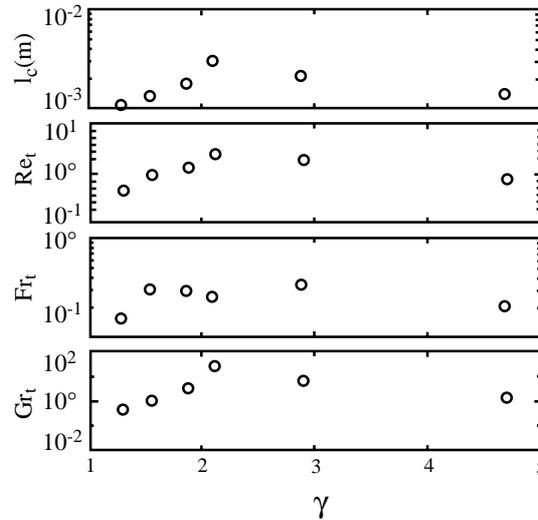
Figure 4. Variation of cycle averaged  $l_c$ ,  $Re_t$ ,  $Fr_t$  and  $Gr_t$  with the parameter  $\gamma$ . The first three panels are extracted from De Silva et al. (1997). The experimental conditions are  $a = 3.1$  cm,  $N = 0.615$  rad/s and  $\alpha = 56^\circ$ .
