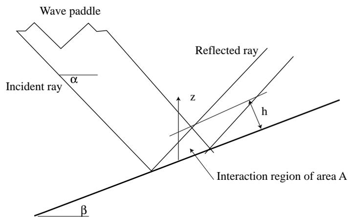
Figure 1. Schematic of internal wave reflection.
