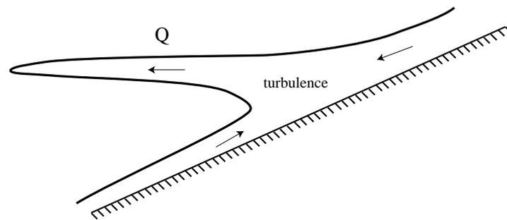
Figure 5. Schematic of the intrusion flow generated by the internal wave breaking process.
