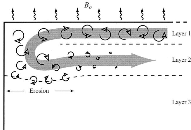
FIGURE 11. Schematic of the dynamics in the vicinity of the basin endwall. The size of the circular arrows implies the relative strength of the turbulence.
