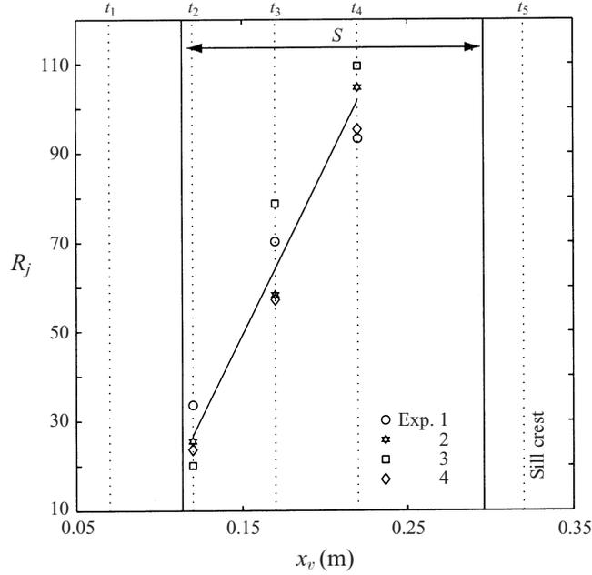
FIGURE 8. The variation of  $R_j$  along the basin for experiments 1–4 (symbols). A solid line, representing a least-squares fit to the measured data, indicates the linear scaling of equation (4.5). Thermistors are labelled along the top.
