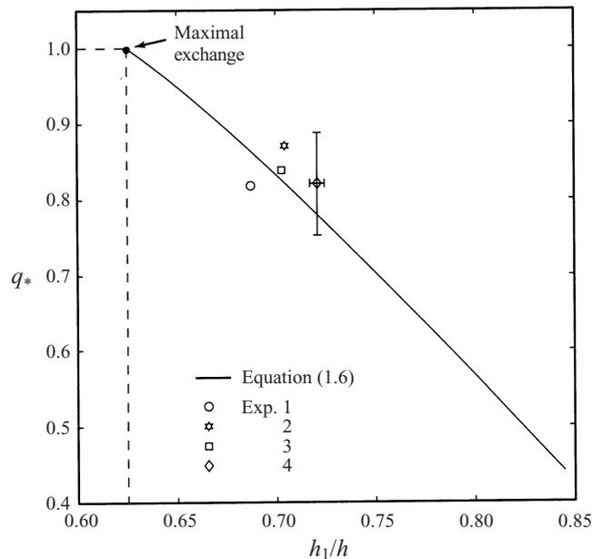
FIGURE 10. The relationship between  $q_*$  and  $h_1/h$  at the sill crest. A solid curve, representing equation (1.6), depicts the relationship over the submaximal range ( $1 > q_* > 0$ ,  $0.625 < h_1/h < 1$ ). Measured experimental values are shown as symbols.
