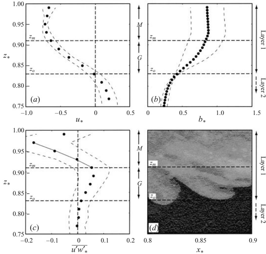
FIGURE 7. Structure of the upper layer shown as profiles of (a) non-dimensional mean horizontal velocity  $u_*$ , (b) non-dimensional mean buoyancy  $b_*$ , (c) non-dimensional Reynolds stress  $u'w'_*$ , and (d) a sample photographic image from experiment 5. Thin dashed lines indicate  $\pm\sigma$ . Note that only the top quarter of the basin depth is shown here so that the structure of the upper layer may be seen clearly. See text for further details.
