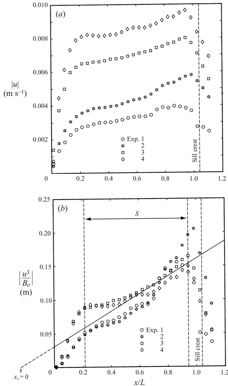
FIGURE 6. (a) Along-basin variation of mean upper-layer horizontal velocity. (b) Variation of the scaling parameter  $|u^3/B_0|$  along the basin. A solid line, fitted to the data within the interior section  $S$ , indicates the scaling associated with equation (3.1) and is extended (dashed line) to the *virtual* origin ( $x_v = 0$ ).
