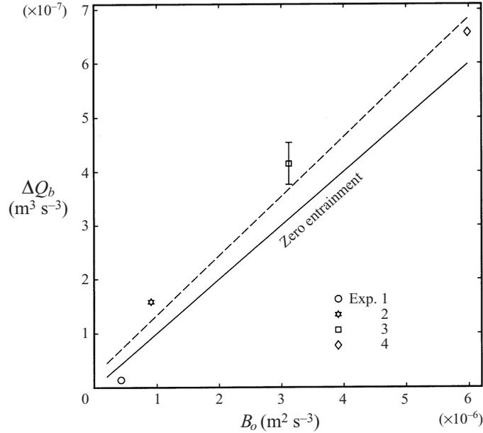
FIGURE 9.  $\Delta Q_b$  between thermistors  $t_2$  and  $t_4$  as a function of the surface buoyancy flux  $B_o$ . The solid line, with slope  $\Delta x$ , represents the expected variation in the absence of entrainment. The dashed line, representing a least-squares linear fit to the measured data (symbols), indicates the actual  $\Delta Q_b$  which includes the contribution from the entrainment flux  $B_e$ .
