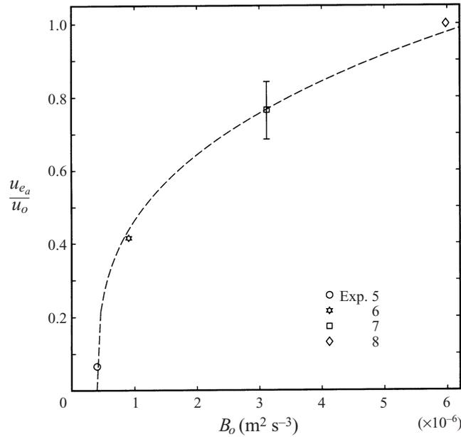
FIGURE 12. Variation of the average entrainment velocity  $u_{ea}$  at the interface between layers 2 and 3, normalized by the maximum measured value  $u_o$ , for experiments 5–8. The  $B_o^{1/3}$  scaling predicted by equation (5.1) is shown as a dashed line.
