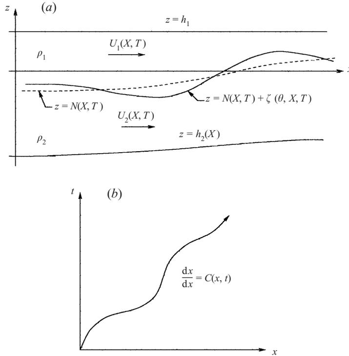
FIGURE 1. Sketch of (a) two-layer model with slow space–time-varying ultra-long wave and variable topography, and (b) the linear characteristic trajectory in the presence of the varying background.
