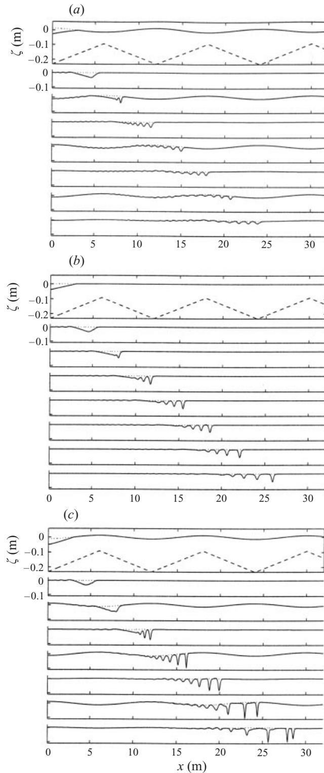
FIGURE 9. Spatial evolution of a long-wave packet at times  $t = 0, 30, 60, 90, 120, 150, 180,$  and  $210$  s for the same conditions described for figure 7. (a) Seiche out of phase with initial condition; (b) no seiche; (c) seiche in phase with initial condition.
