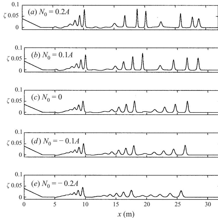
FIGURE 2. Effect of changing the amplitude and the phase of the background seiche on the evolution of a long-wave packet. Seiche wave amplitudes at  $x = 0$  are noted on the respective panels. Each panel contains the spatial structure of the packet at the times  $t = 0, 50, 100, 150$  s. All simulations have  $h_2/H = 0.2$ ,  $\Delta\rho/\rho_2 = 0.02$  and  $L = 6$  m.
