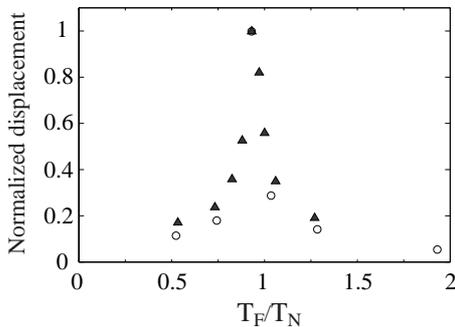
Figure 4: Normalized interface displacement recorded at position 1 as a function of the dimensionless forcing period  $T_F/T_N$  for  $S = 0.5$  (filled triangles) and  $S = 0.25$  (circles). Steady state interface displacements were measured after 20 forcing events and are normalized by the interface displacement at resonance  $T_F/T_N = 0.94$ .
