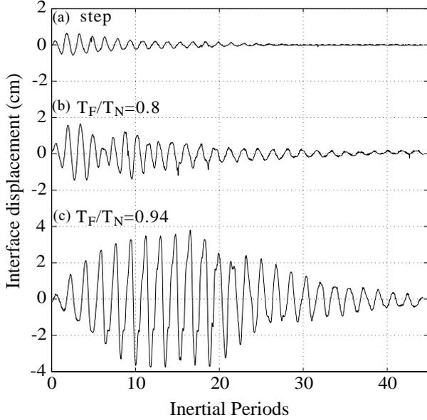
Figure 3: Time series of interface displacement recorded at position 1 for  $S = 0.5$  subject to (a) a step forcing (b) 10 forcing events with  $T_F/T_N = 0.8$  (c) 10 forcing events with  $T_F/T_N = 0.94$ .
