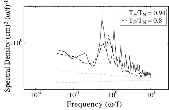
Figure 5: Power spectra of the interface displacement recorded at position 1 for  $S = 0.5$  subject to 20 forcing events with  $T_F/T_N = 0.8$  and  $T_F/T_N = 0.94$ . The solid vertical lines indicate the frequency of the natural modes of the basin (see figure 2 (b)) which satisfy the imposed initial condition. Spectra were smoothed in a similar manner to figure 2
