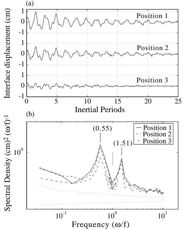
Figure 2: (a) Time series of the interface displacement for  $S = 0.5$  following a step forcing. (b) Power spectra of the interface displacements shown in (a). The wave frequency  $\omega$  is scaled by  $f$  with the dashed vertical line identifying the inertial frequency  $f$ . Spectra have been smoothed in the frequency domain to improve confidence, with the 95% confidence level is given as the difference between the two dotted lines at a prescribed frequency [3].
