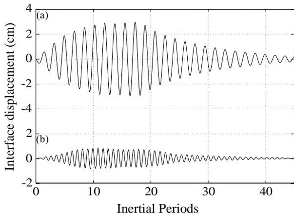
Figure 6: Bandpass filtered time series of interface displacement recorded at position 1 for  $S = 0.5$  subject to 10 forcing events with  $T_F/T_N = 0.94$  for (a) the Kelvin wave, (b) first harmonic of the forcing frequency.
